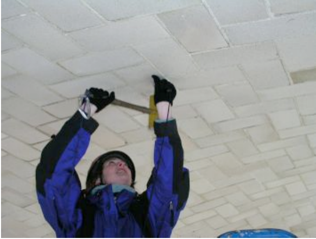
Hammer-sounding a Guastavino tile ceiling
